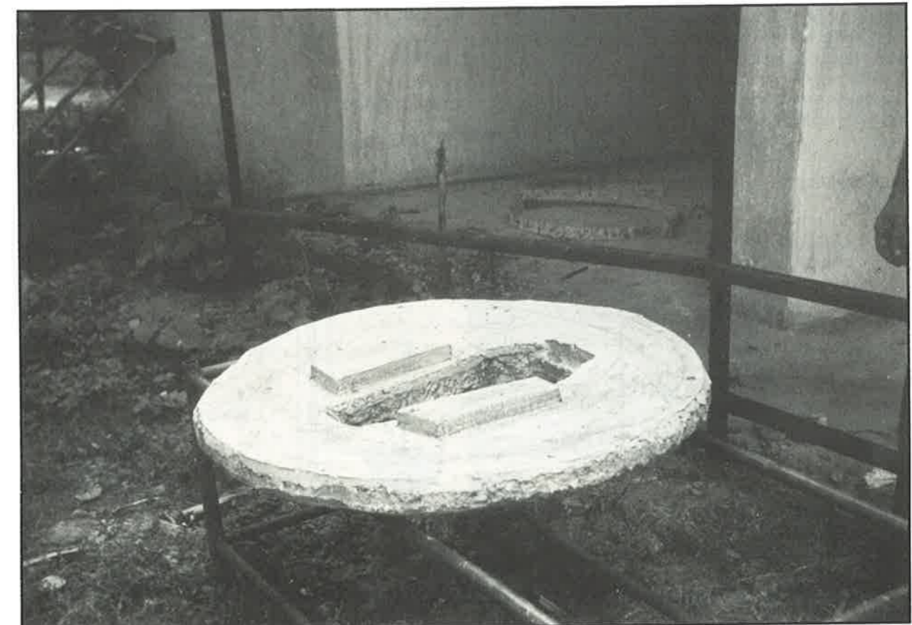
Below: Local production of latrine slabs for sale to householders
